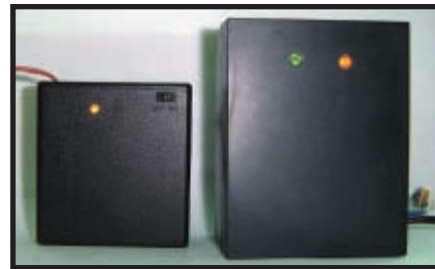
Photo 2 —A battery-operated frequency meter (left) only needs to be near the base unit in order for them to communicate. The glowing yellow and orange LEDs indicate that data are being transferred between the two.
